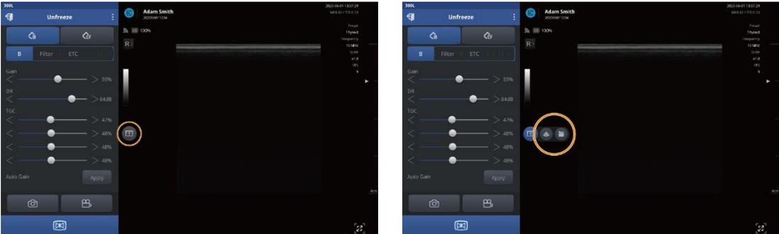
The reference sources for comparison, such as recorded images, videos, or freeze mode will be displayed on the left screen while in dual screen.
